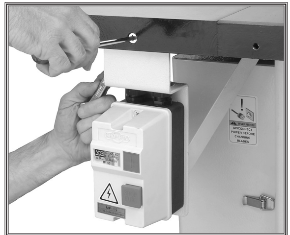
Figure 20. Attaching switch to extension wing.
